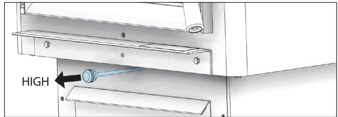
After the first high burn load and the stove is well warmed up, adjust the unit as needed for a medium or low burn setting. For a medium burn, once the high burn fuel load is burned down to an established coal bed, rake and level the coal bed. Load the unit with 33 lbs of cordwood and close the door immediately. Leave the air control fully open (in the “HI” position) for 8 minutes. After 8 minutes push in the air control to the medium position (midway between the “Low” and “Hi” position).
