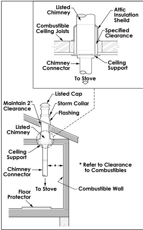
Ensure that a masonry chimney meets the minimum standards of the National Fire Protection Association (NFPA) by having it inspected by a professional. Make sure there are no cracks, loose mortar or other signs of deterioration and blockage. Be sure to the chimney cleaned before the stove is installed and operated. When connecting the stove through a combustable wall to a masonry chimney, special methods are needed.
