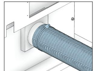
Slide the hose clamp over the aluminium flex pipe. Then slide the flex pipe over the air intake tube of the stove. Next tighten the hose clamp over the end of the aluminium flex hose.
