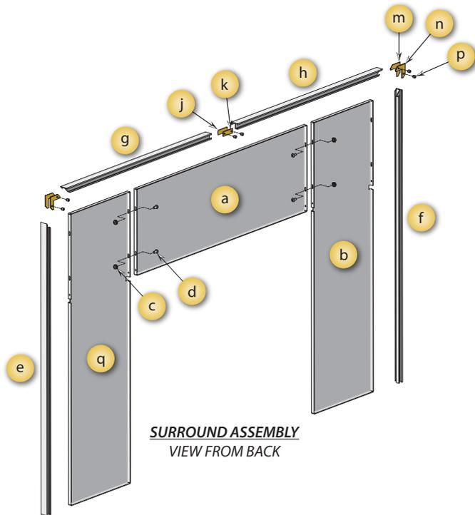
1. Lay pieces face down on carpet or other soft surface to protect finish during assembly. The Surround consists of two side panels, a top panel, and a decorative trim frame.
