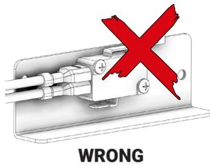
**ENSURE THE WIRES ARE CONNECTED TO THE BOTTOM TWO PRONGS OF THE HOPPER SWITCH AS SHOWN.**
