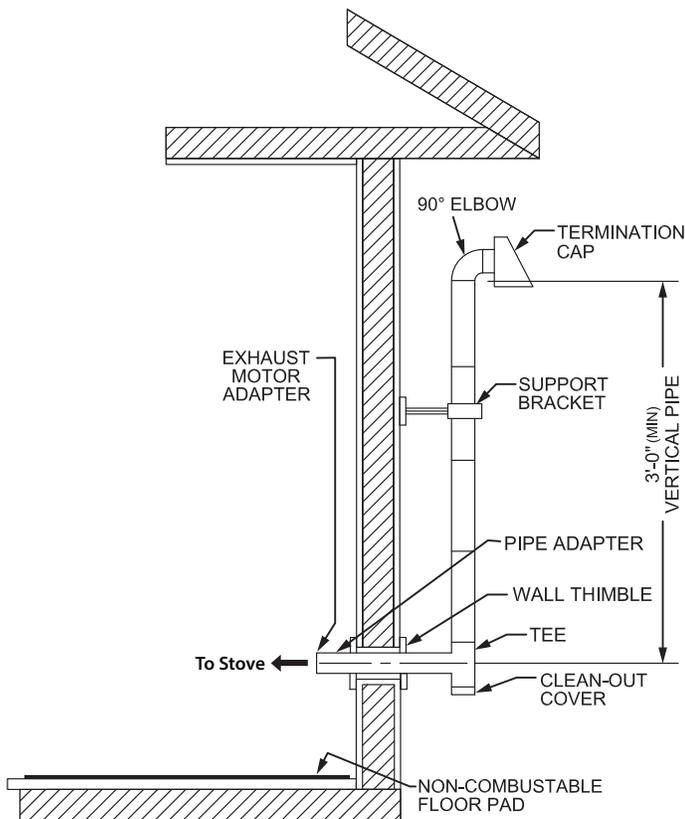
Canadian installations must conform to CAN/CSA-B365. To vent the unit through the wall, connect the pipe adapter to the exhaust motor adapter. If the exhaust adapter is at least 18" (457 mm) above ground level, a straight
