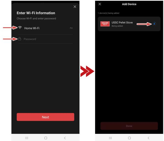
5. Select “Add Device”. Note: Access to location and Bluetooth is required while using the app.
