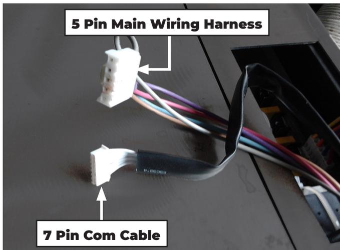
2. Unpack the top mount controls and ensure that all wires are securely attached.
