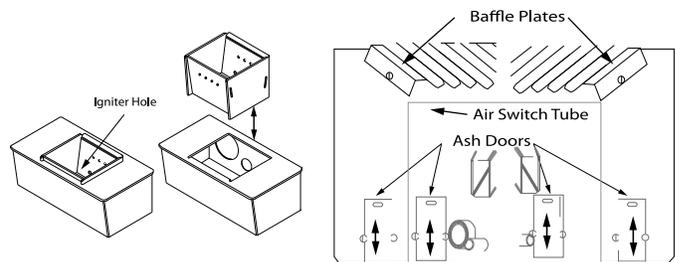
4. Empty ashes from the inner section and scrape with cleaning tool; make sure holes are not plugged.
