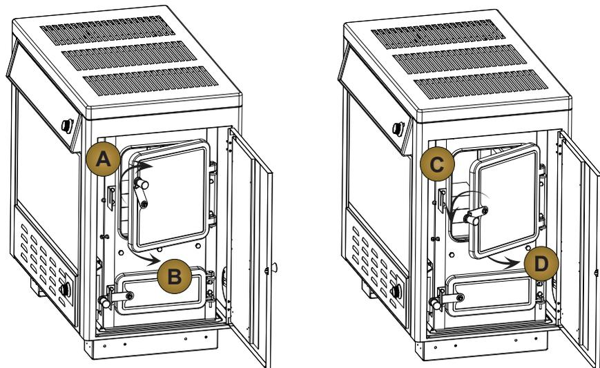
NOTE: During opening and closing of the feed and ash doors of this heater, it may seem that the fit of the door is "too tight". As the heater is fired, the gasketing "settles" or "seats" itself in the door. The tight fit at the factory and before the heater's initial firing is to insure a good seal after the gasketing "settles".
