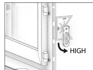
After the first high burn load and the stove is well warmed up, adjust the unit as needed for a medium or low burn setting.
