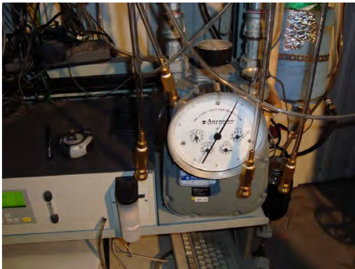
Picture 8: Reference dry gas meter
