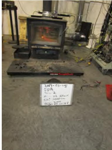
Medium load burning in the stove run 2.1
