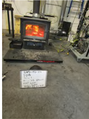
Minimum load burning in the stove run 1.2
