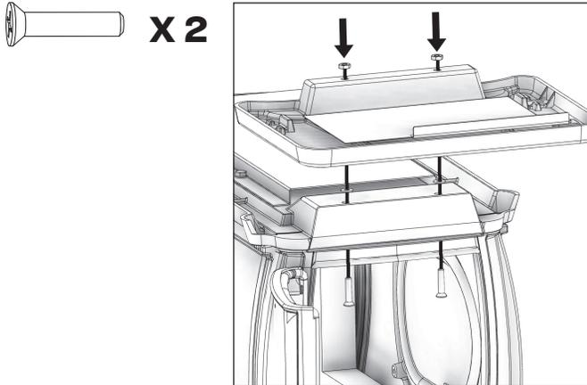
8. Carefully lift the stove upright and place in the desired location. Align the holes on the flue collar to the holes on the stove and attach using (2) two M6 X 15 screws.
