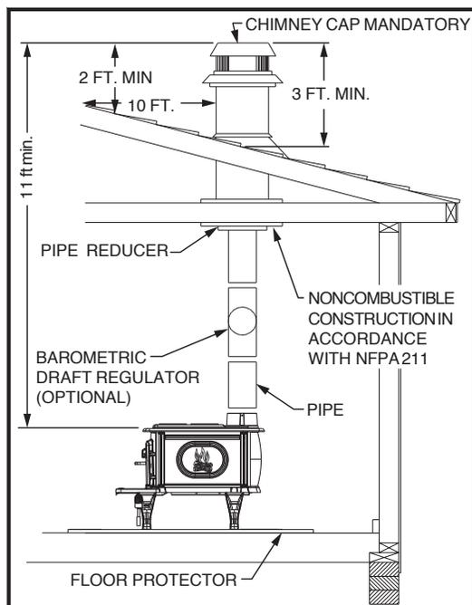
leak smoke into the room through appliance and chimney connector joints. An uncontrollable burn or excessive temperature indicates excessive draft.
