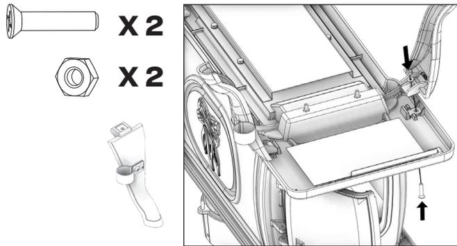
9. Lower the feed door into position while aligning hinge pins.
