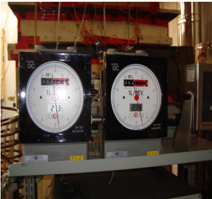
Picture 11: Dry gas meter
