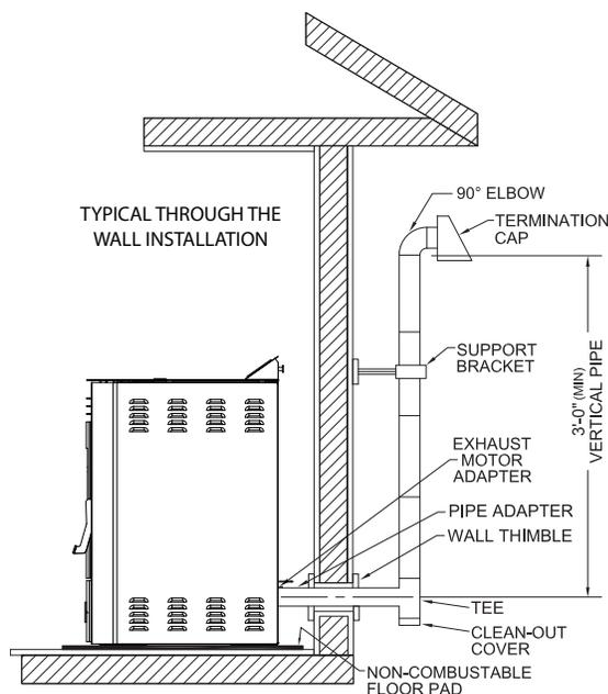
Canadian installations must conform to CAN/CSA-B365. To vent the unit through the wall, connect the pipe adapter to the exhaust motor adapter. If the exhaust adapter is at least 18" (457 mm) above ground level, a straight section of pellet vent pipe can be used through the wall.
