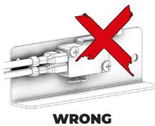
**Ensure the wires are connected to the bottom two prongs of the hopper switch as shown.**
