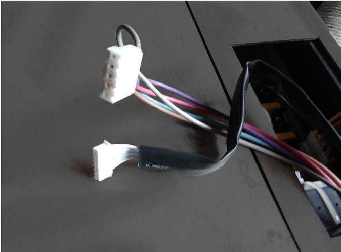
2. Unpack the top mount controls and ensure that the wiring harness shown is attached securely.
