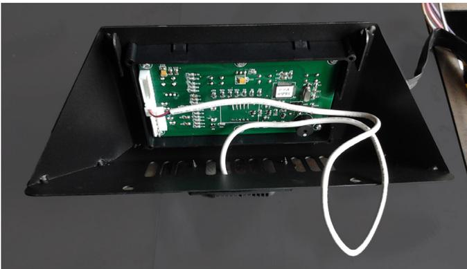
3. Connect the factory installed wiring harnesses to the control panel as shown.
