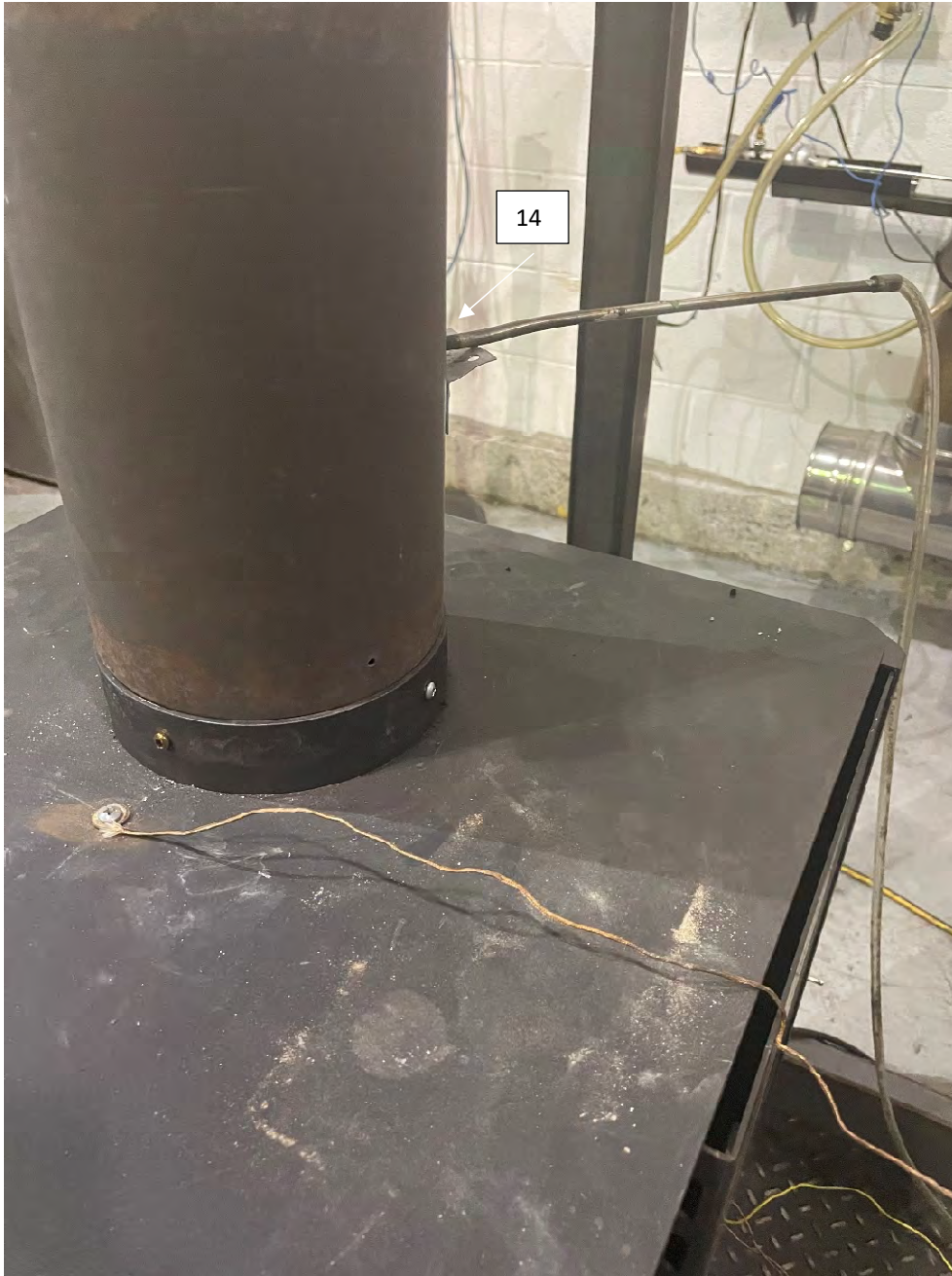
14 : Draft sampling port located 6 in. from the flue outlet
