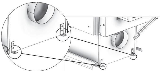
In addition to the previously detailed installation requirements, the heater must be electrically grounded to the steel chassis of the Mobile Home/Transportable Buildings with 8 GA copper wire using a serrated or star washer to penetrate paint or protective coating to ensure grounding.
