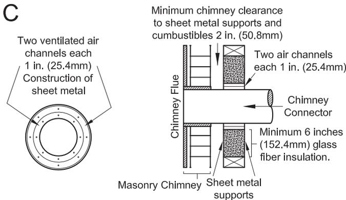
**METHOD D - 2" (51 mm) Clearance to Combustible Wall Member:** Start with a solid-pak listed factory built chimney section at least 12" (304 mm) long, with insulation of 1" (25.4 mm) or more, and an inside diameter of 8" (2 inches [51 mm] larger than the 6" [153 mm]
