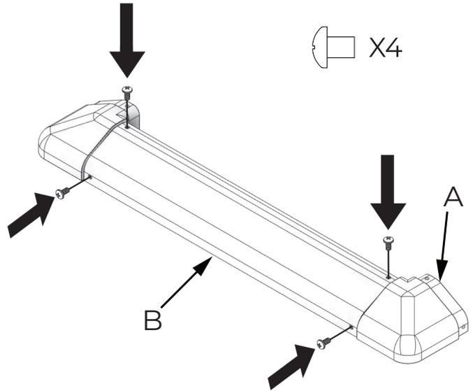
2. Attach the side skirting sections (C & D) to the corner pieces and secure with four (4) truss head screws.
