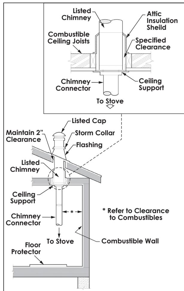
When a metal prefabricated chimney is used, the manufacturer’s installation instructions must be
