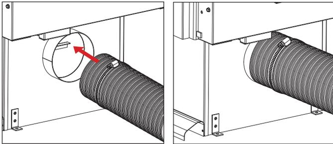
Slide the hose clamp over the aluminium flex pipe. Then slide the flex pipe over the air intake tube of the stove. Next tighten the hose clamp over the end of the aluminium flex hose.
